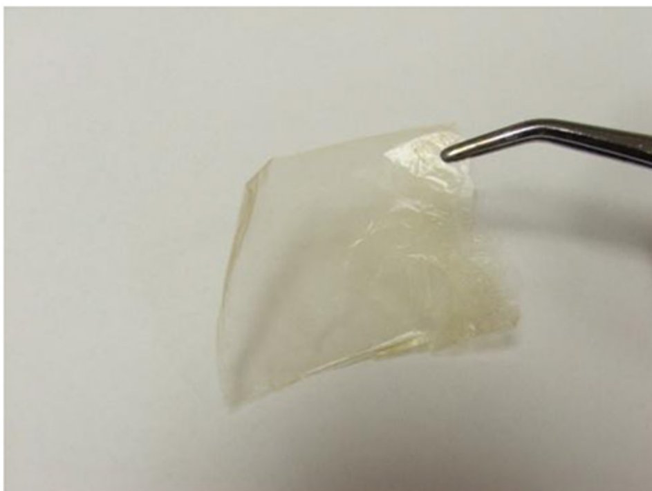
Figure 7. A free-standing film of NC-PDDA-HMWL obtained after 250 deposition cycles. The free-standing films were obtained after dissolving the cellulose acetate substrate in acetone.
