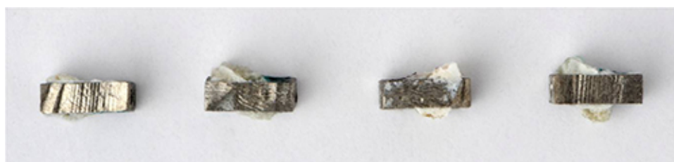
Figure 10. Breaking patterns of cortical arches around the implants following mechanical testing.
