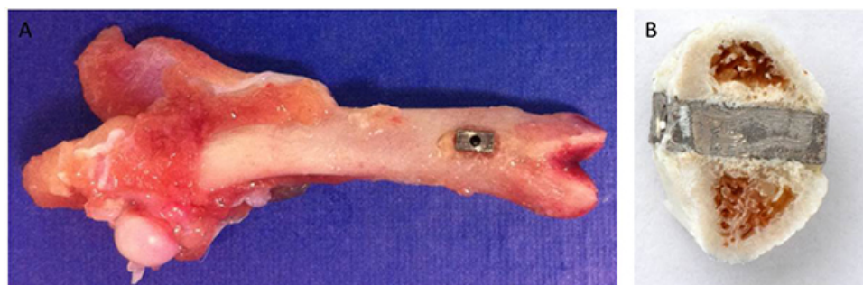
Figure 4. (A) Femora were harvested from sacrificed animals. The rectangular implant is visible in the distal femur. (B) Final test specimen with both a medial and a lateral arch on either side of the implant.
