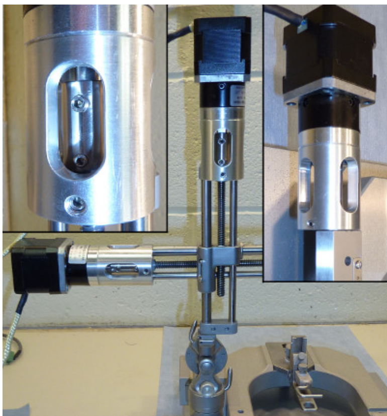
Figure 4. Assembly diagram for attaching the motors/couplers to the collars/stereotaxic arm.
