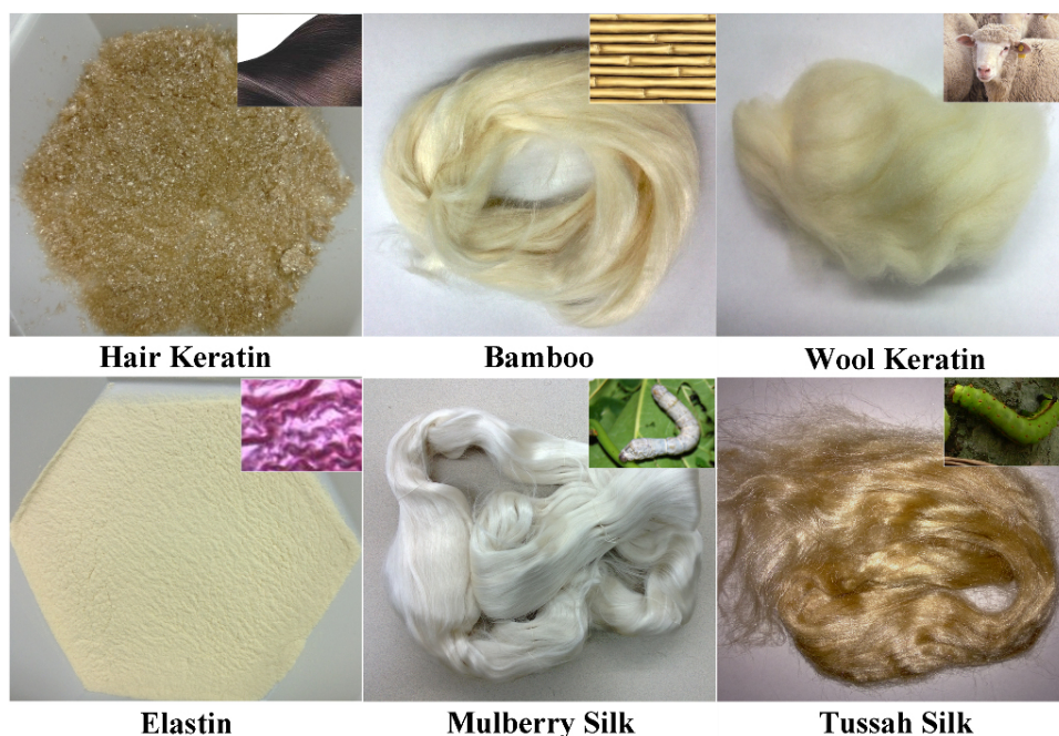
Figure 1. Raw materials of various structural proteins that are commonly used in our laboratory for designing protein-based materials, including silks from different worm species, keratins from hairs and wools, elastins from different tissues, and various plant proteins.
