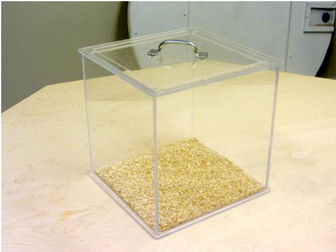
Figure 1. Equipment set up for the inchworming experiment. Equipment set up for the inchworming experiment. A 30 cm cube Plexiglas box is set on a table in front of an infrared zoom camera positioned at a 45° angle. The bottom of the enclosure is covered fully with an even layer of at least 1 inch of sawdust.
