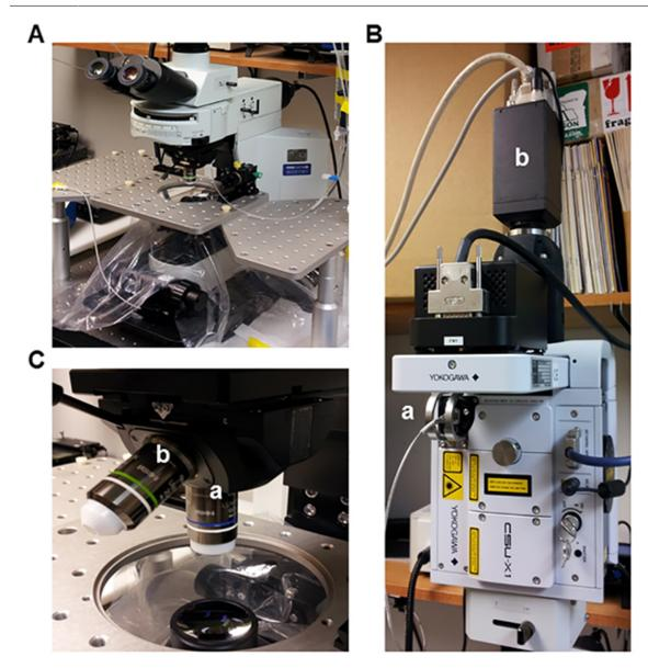
Figure 2. Spinning disc confocal microscope for imaging of Ca<sup>2+</sup> signals. A) Upright microscope used for calcium imaging. B) (a) Confocal spinning disc unit with an (b) intensified charge coupled device camera. C) Immersion objectives (a) 63X (NA = 1) and (b) 20X (NA = 0.5) used for imaging. Click here to view larger image.
