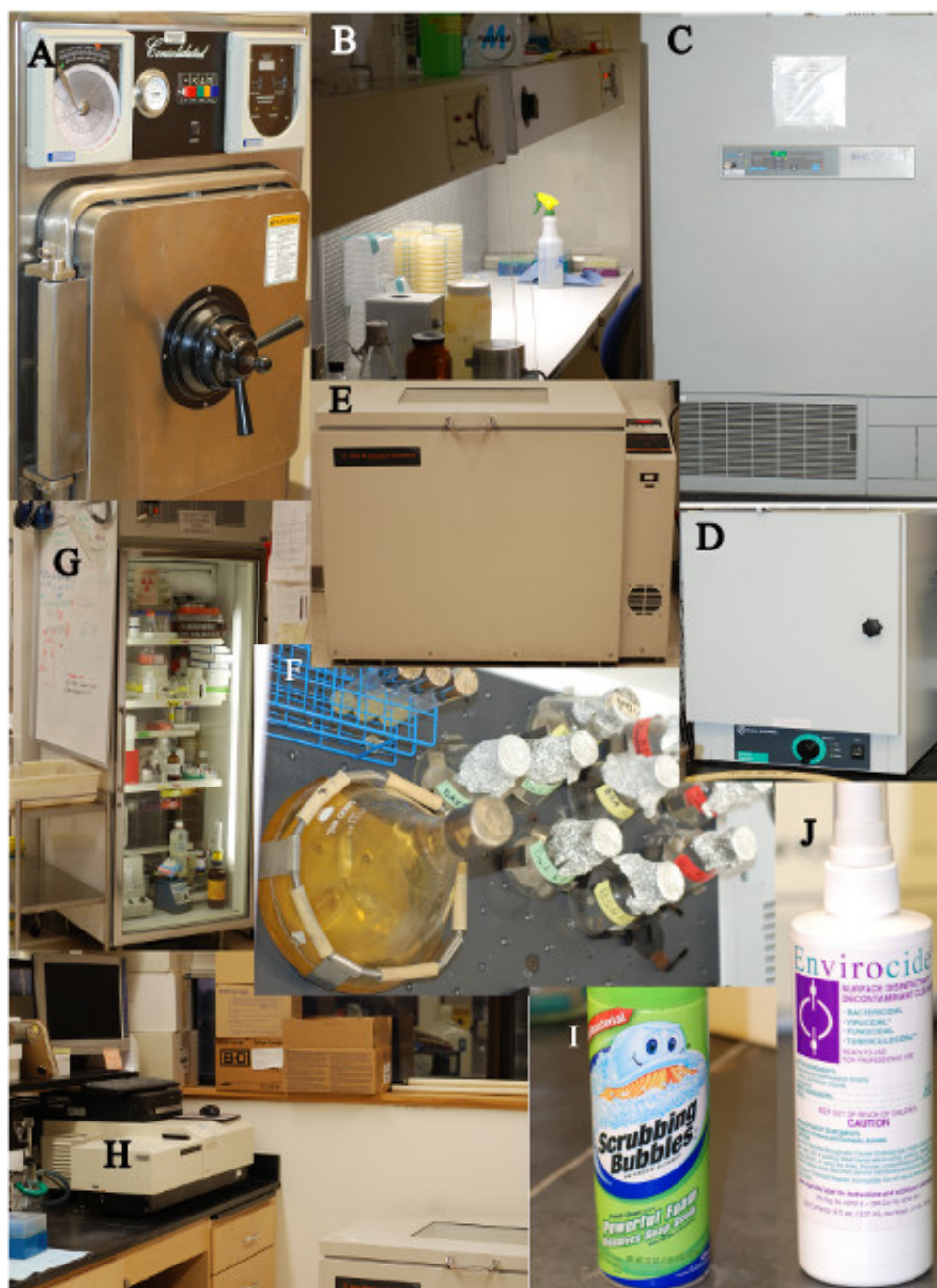
Figure 2. Some of the equipment and material necessary for performing phage display. Sterile technique requires access to both: A) an autoclave and; B) a laminar flow hood. Phage libraries and BLT5403 bacterial stock require -80^{\circ}\text{C} temperatures for prolonged storage C) Growing phage and bacteria requires, D-F) 37^{\circ}\text{C} incubators, one of which, E-F) is capable of growing liquid cultures (orbital). Optimizing the experiment through color coding, F) minimizes mistakes. BLT5403 cells for titering can be stored for up to one week, G) at 4^{\circ}\text{C} . Optimizing the placement of the, H) spectrophotometer for following cell densities next to the orbiting shaker can save time. Frequently treating surfaces and pipettes with, I) powerful detergent and J) Envirocide, can help to minimize the risk of viral contamination. Click here to view larger image.
