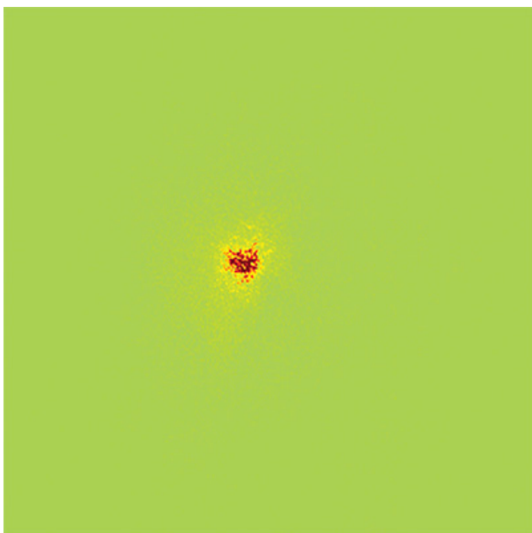
Figure 4. Intensity Profile. Intensity profile of the propagated beam after 5 cm of propagation. The width of the image is 250 \mu\text{m} .
