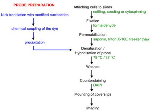
Figure 1. Workflow for probe labeling and DNA FISH. Probe preparation is shown in blue. DNA FISH procedure is shown in black with details given in green.
