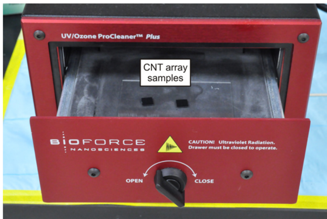
Figure 3. A commercial UV/ozone cleaner used to render CNT arrays hydrophilic by functionalizing them with oxygenated functional groups.
