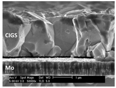
Figure 1. SEM image of a CIGS layer on Mo coated soda lime glass substrate.
