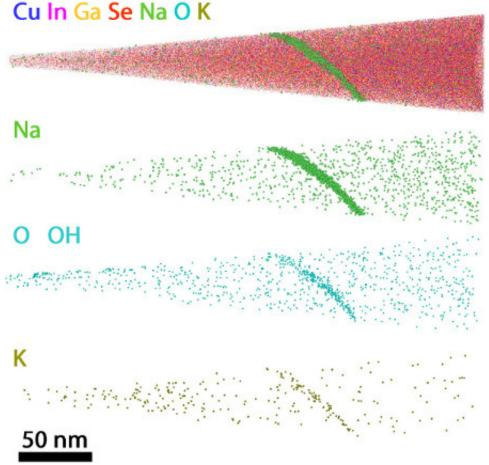
Figure 3. 3D APT maps of Cu (blue), In (pink), Ga (yellow), Se (red), Na (green), O and OH (light blue), and K (khaki). These 3D maps directly show Na, K and O segregation at a HAGB (28°-<511><sub>cub</sub>), which was analyzed by EBSD and TEM prior to the APT analysis.
