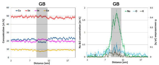
Figure 4. (a) Cu, Se, Ga, In and (b) Na, K, O concentration depth profiles through the GB shown in Figure 3. The sampling box used to build these profiles is 32 x 32 x 0.3 nm<sup>3</sup>. Bars give the statistical errors (2σ). Click here to view larger figure.
