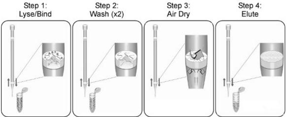
Figure 1. The TruTip extraction process and work flow, regardless of the liquid handling system. Other sample preparation or liquid handling steps can be incorporated into automated routines depending on the capabilities of the specific liquid handling instrument and software.
