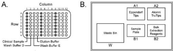
Figure 2. (A) Eppendorf epMotion 5070 sample plate layout. (B) Arrangement of reagents/consumables on the Worktable. The sample plate can be configured for up to 24 samples (columns 1, 5 and 9, respectively), although the epMotion will only process a maximum of 8 samples simultaneously. Click here to view larger figure.
