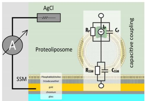
**Figure 1.** Adsorption geometry of proteoliposomes on the SSM. The SSM is formed on a sensor chip, a structured gold coated glass slide. To measure electrogenic reactions of membrane proteins, proteoliposomes or membrane fragments are adsorbed to the SSM. The two membranes form a capacitively coupled system. This is why only transient currents are detected.
