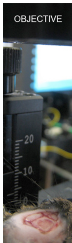
Figure 2. OCT imaging of TSCW in vivo . A mouse model with a thinned-skull is fixed in a stereotactic frame under the objective for OCT imaging in vivo .
