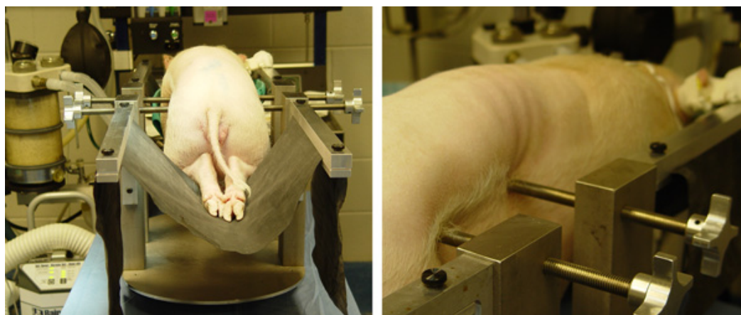
Figure 1. Table Positioning for Procedure. Animals are placed into a prone position on a frame custom designed to mimic patients positioning on a Jackson spinal surgical table. The frame utilizes adjustable slings that are placed under the chest and pelvis of the animal, allowing the abdomen to hang free and, therefore, minimizing pressure on the abdomen and chest and consequent epidural venous bleeding. The frame also provides external immobilization of the spine for the procedure.
