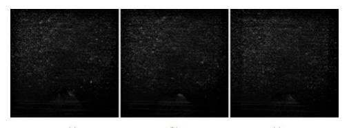
(a) (b) (c) Figure 5. From left to right: Raw refocused SAPIV images at depths (a) Z = -5.9 mm, (b) -10.6 mm and (c) -15.3 mm.
