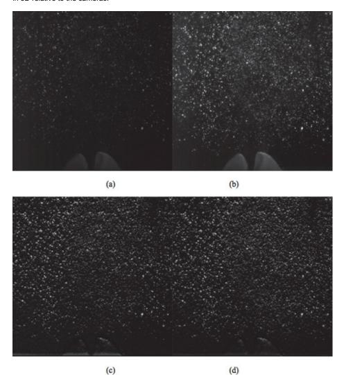
Figure 4. Raw images of the particle field viewed from camera #6 at t<sub>1</sub> and t<sub>2</sub> (a & b). Same images after pre-processing (c & d).
