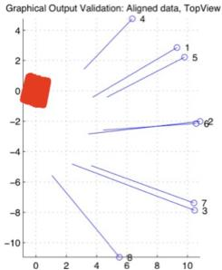
Figure 3. Topview of camera setup from multi-camera self calibration output. Cameras 1-8 are located with numbers and circles, with their general viewing direction indicated by a line. The red blob near the origin is actually 400+ points from the calibration grid at each Z depth plotted in 3D relative to the cameras.
