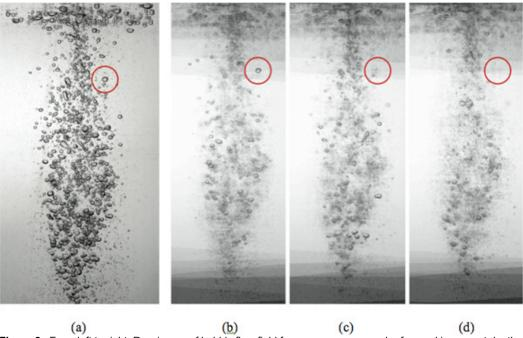
**Figure 8.** From left to right: Raw image of bubbly flow field from camera array and refocused images at depths **(b)** Z = -10 mm, **(c)** 0 mm and **(d)** 10 mm. The circle highlights a bubble that lies on the Z = -10 mm depth plane, and disappears from view on other planes. Details of the bubble experiments can be found in  $^4$ .
