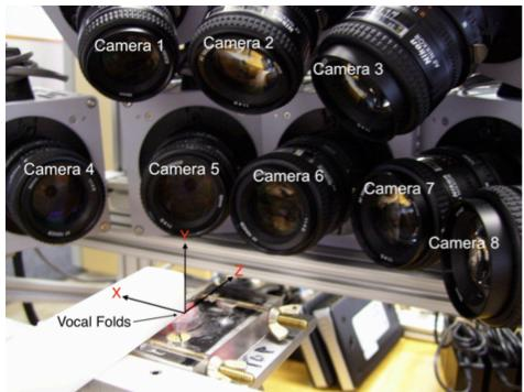
Figure 1. Image of cameras and vocal folds with labels and coordinate system.
