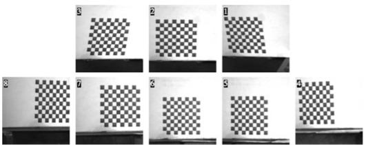
Figure 2. Calibration grid at Z = 0 mm as seen from all 8 cameras.
