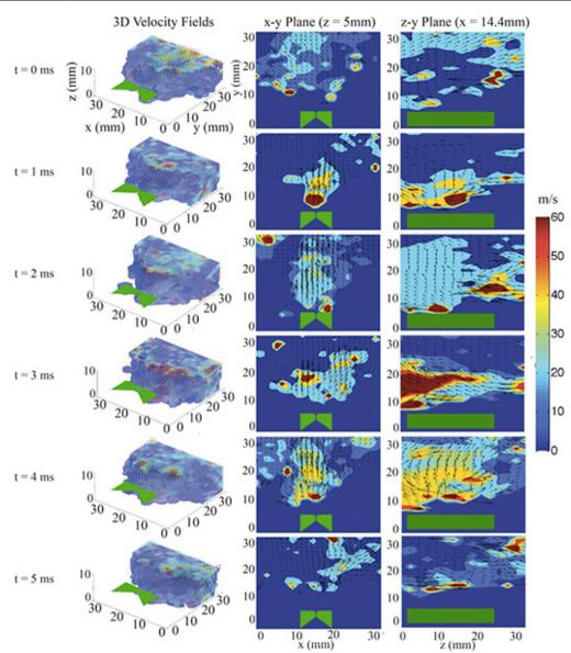
**Figure 7.** Three-dimensional vector field of the jet created by synthetic vocal folds for 6 time steps. The left hand side shows an isometric view of the entire 3D velocity field. Cuts of the x-y and y-z planes are made through the center of the vocal fold as indicated above each column.
