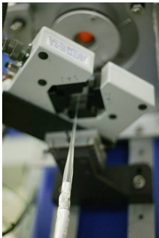
Figure 16. + Drop-down preform section.
