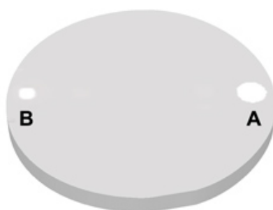
Figure 3. Schematic of holes that should be drilled into the lids the galvanotaxis chamber and the culture medium reservoirs. The 7 mm diameter holes in both lids are used to insert the agarose gel tubes. The 4 mm diameter holes in the lid of the galvanotaxis chamber is used to measure the electric potential directly across the central trough using a voltmeter. The 4 mm diameter hole in the lid of the culture medium reservoir is to allow the Ag/AgCl electrode to protrude from the lid of the dish for connection to the power supply.
