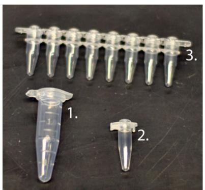
Figure 4. Sterile tubes used for PCR. (1.) 1.8 ml tube (2.) 0.2 ml individual thin walled PCR tube, (3.) 0.2 ml strip thin walled PCR tubes and caps.
