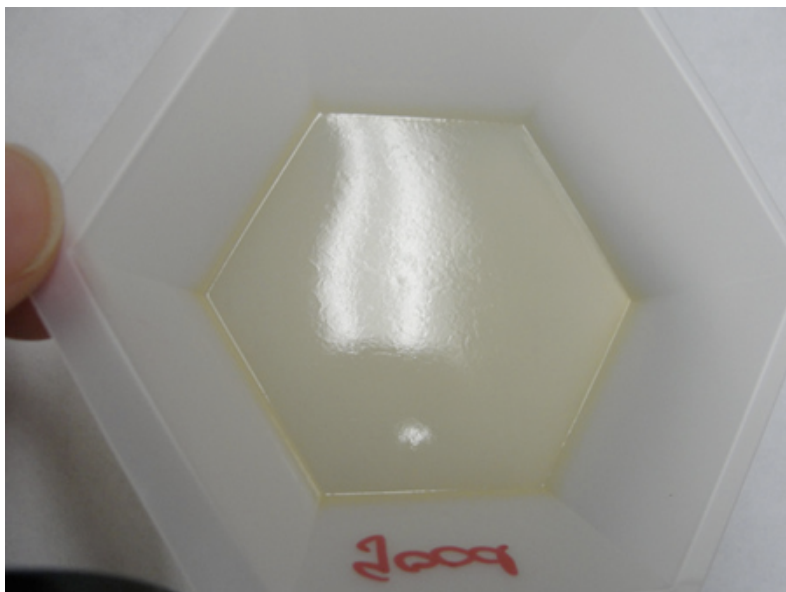
Figure 2. Optical photograph of initial co-cast films of Nafion and TBAB. Slow drying yields a transparent, light brown film covering the bottom of the weighing tray.
