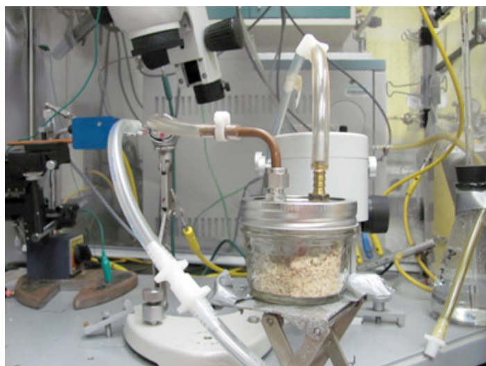
Figure 5. Small modified vessel containing a sample matrix and associated volatiles to be puffed across A. transitella antennae.
