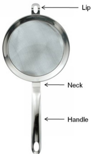
Figure 7. Strainer with wire mesh and stainless steel handle is used to retrieve cryovials from Dewar. If the handle is not provided with a slot, drill with carbide bit will be required for drilling a hole.
