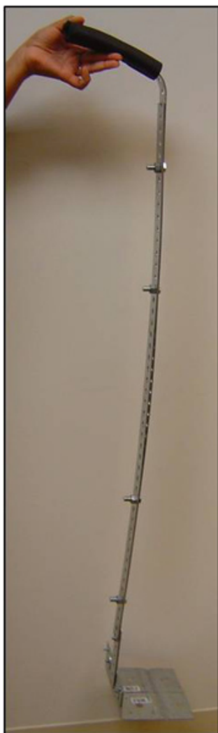
Figure 5. The flat base consisting of strong-ties and T strap is then secured at one end of the slotted plate. The larger hole on the remaining corner of T strap is aligned with the slot on the flat plate and fastened using hex bolt and nut. This device can be now used to retrieve cryoboxes from Dewar.
