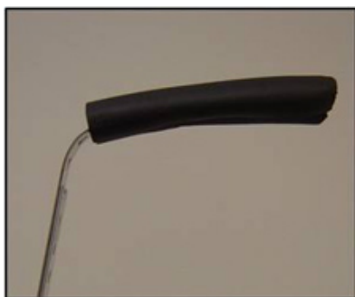
Figure 6. One end of the slotted flat plate is bent using pliers and covered with foam to provide better grip especially for deep Dewars, as shown in this case.
