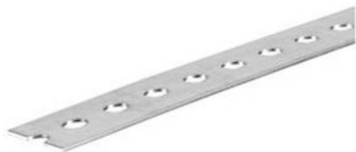
Figure 4. Slotted flat plate is used as the handle. Length of the slotted plate depends on the depth of the Dewar. In this case, 4 feet of slotted plate was used. The thickness of slotted plate is critical since thin slotted plates (<14 gauges) make the device flimsy while retrieving samples from liquid nitrogen filled Dewar.
