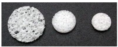
Figure 1. Dehydrated PVA sponge disks in three different sizes.
