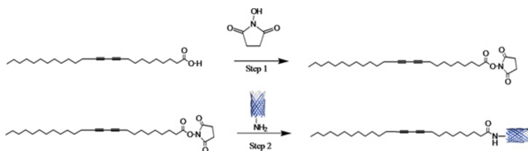
Figure 2. Reaction scheme for the PCDA-NHS synthesis (step 1). Reaction of PCDA-NHS to the amine substituent of proteins (step 2). Step 2 is the basis of binding of lysine residue of proteins to the carboxylic acid of PCDA monomer. Click here to view larger figure.
