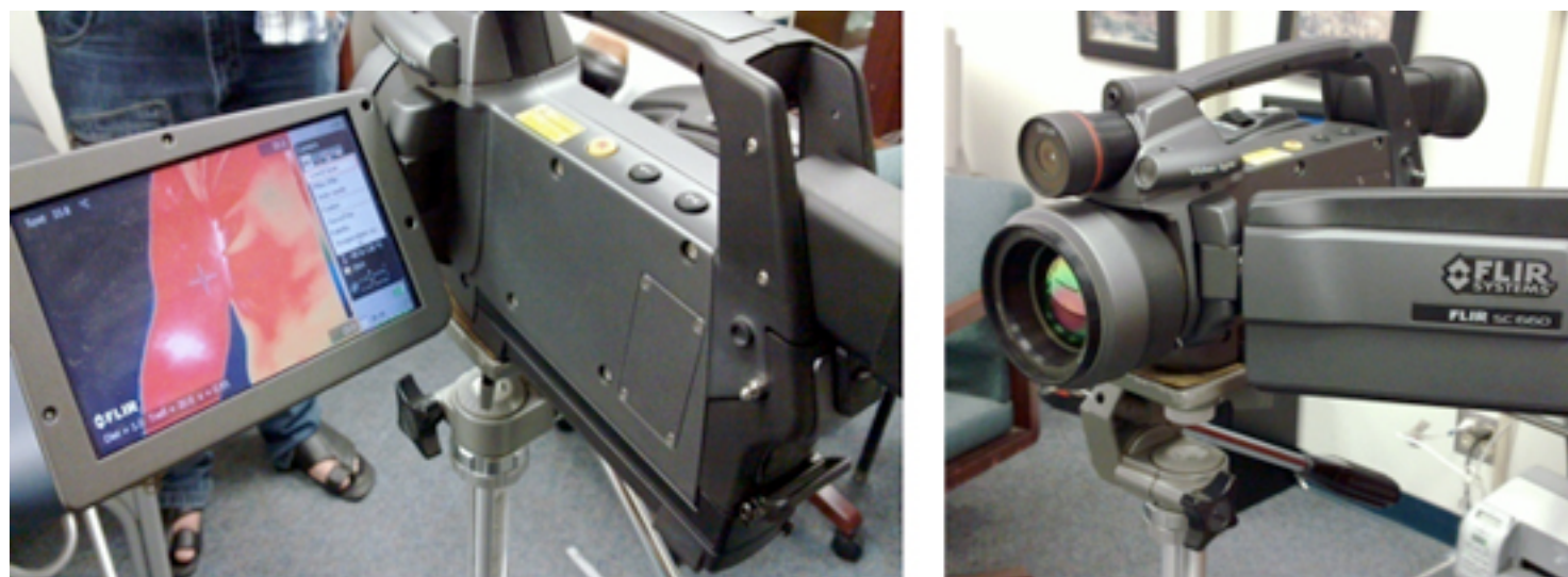
Figure 8. The IR thermal camera used for this investigation (FLIR 660).
