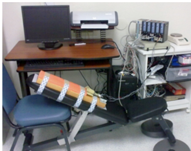
Figure 10. A) The BioPac Modules used for measuring the muscle strength. B) The strain gauge device fixed to a 45° angled bench and hooked to the BioPac system.
