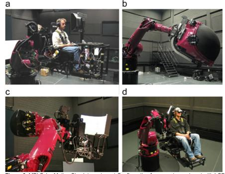
**Figure 3.** MPI CyberMotion Simulator setup. a) Configuration for current experiment with LCD display. b) Configuration for experiments requiring an enclosed cabin with front projection stereo display. c) Front projection mono display. d) Head mounted display.
