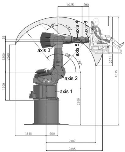
Figure 1. Graphical representation of the current MPI CyberMotion Simulator work space.
