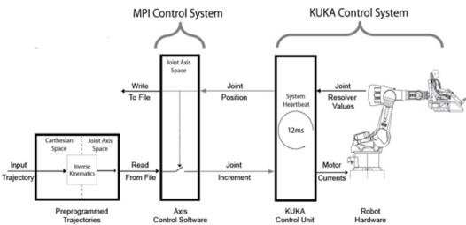
Figure 2. Schematic overview of the open-loop control system of the MPI CyberMotion Simulator. Click here for larger figure.
