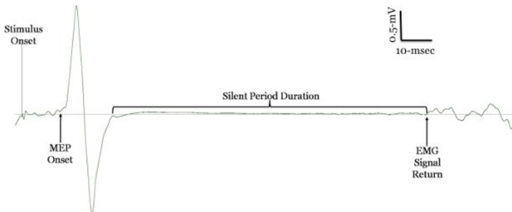
Figure 5. TMS during a contraction: motor evoked potential & silent period. The silent period is observed when a subject performs a slight contraction and a single stimulus is applied to the motor cortex. The first part of the silent period is due to spinal cord inhibition and the latter part is attributed to cortical inhibition, specifically GABA B receptors. There is no consensus way to quantify the duration of the silent period, but our findings indicate that either defining it from stimulus onset or MEP onset to the return of the voluntary interference electromyogram signal is the most reliable 15 .
