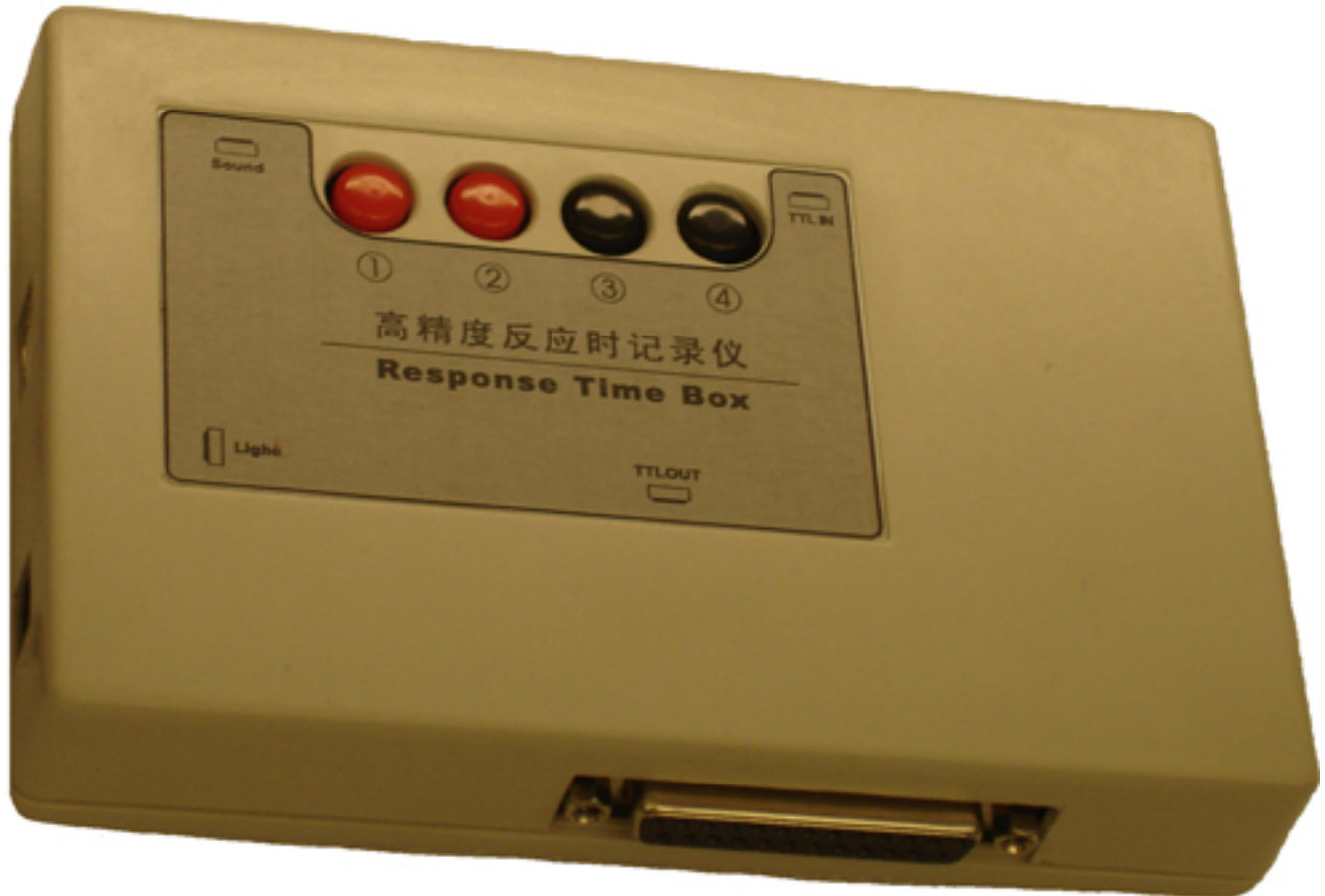
Figure 4. Picture of an RTbox. It has a USB-B port, a light input port, a pulse/sound input port, an external button input port, and a TTL output port.
