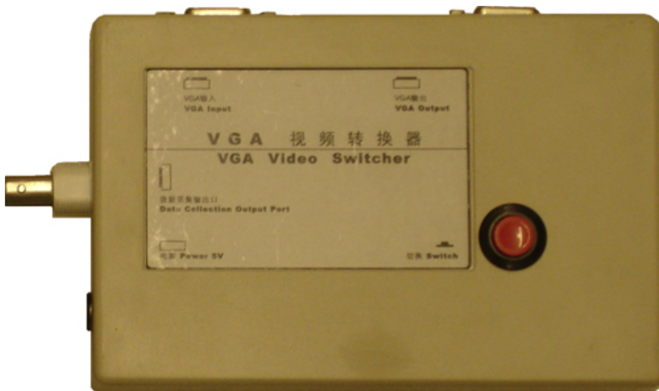
Figure 1. Picture of a video switcher. It has VGA input and output ports (both female), a button to switch between two display modes, and a trigger output port.
