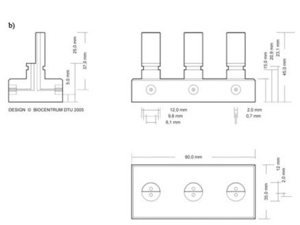
**Figure 2.** Schematic drawing of flow cell and bubble trap<sup>2</sup>. Detailed description of the dimensions used for the production of a) flow cell b) bubble trap, DTU Systems Biology. Reprinted with permission of John Wiley & Sons, Inc. (DTU Systems Biology was formerly entitled Biocentrum, as depicted in the figure)
