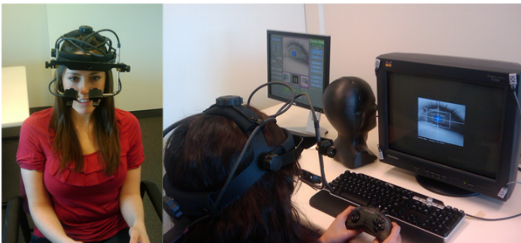
Figure 1. Example of a head-mounted video-based eye tracker (left) and the display and host PCs (right). Note that the display monitor in front of the participant shows the location of the pupil (blue dot with crosshair) and corneal reflection (yellow dot with crosshair) to aid in camera setup.
