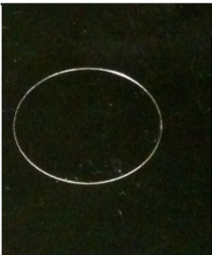
Figure 1A. Improperly washed coverslip. Following addition of APTMS, coverslip was washed for 1-2 minutes before addition of the glutaraldehyde solution. A precipitate forms on the coverslip that has not been washed according to the steps outlined in Procedure.
