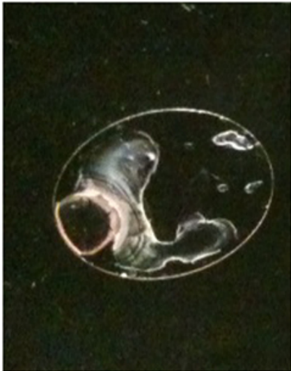
Figure 1A. Improperly washed coverslip. Following addition of APTMS, coverslip was washed for 1-2 minutes before addition of the glutaraldehyde solution. A precipitate forms on the coverslip that has not been washed according to the steps outlined in Procedure.
