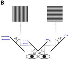
**Figure 3:** Mirror stereoscope. (A) An observer looking through a commercially-available mirror stereoscope. (B) A schematic representation of a mirror stereoscope. Solid lines represent mirrors. Dotted lines represent line of vision, and blue arrows represent possible adjustments to either the location (straight arrows) or angle (curved arrows) of mirrors. Each type of arrow is only shown on one side for simplicity, but the same adjustments can be made on both sides.
