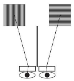
**Figure 6:** Prism goggles. Each prism lens bends light, causing stimuli that are physically side-by-side to appear to be in the same spatial location. Note that a divider is required to prevent additional lines of vision.
