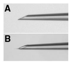
**Figure 1.** Shapes of the transplantation needle tips. A. The beveled opening of the tip of a needle was free of debris after hydrofluoric acid washes. B. A pointed end was generated at the needle tip.
