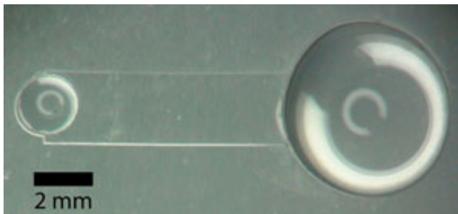
Figure 1. PDMS microfluidic device with one inlet, left, and one outlet, right. Please click here to see a larger version of figure 1.
