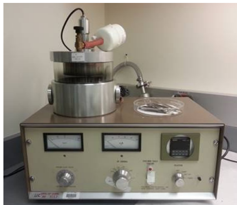
Figure 2: Gold-Palladium sputter coater showing the sample chamber (silver vessel on top) and vacuum (left) and current (right) gauges. In this model, a current of 2 mA is used with a chamber vacuum of .1 torr, which is kept constant using an Argon leak valve.
