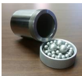
Figure 1: Stainless steel vial with two different sizes of balls.
