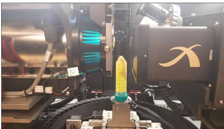
Figure 2: Mouse spine suspended in agarose gel inside thin-walled plastic tube sitting on sample stage of micro-CT system.
