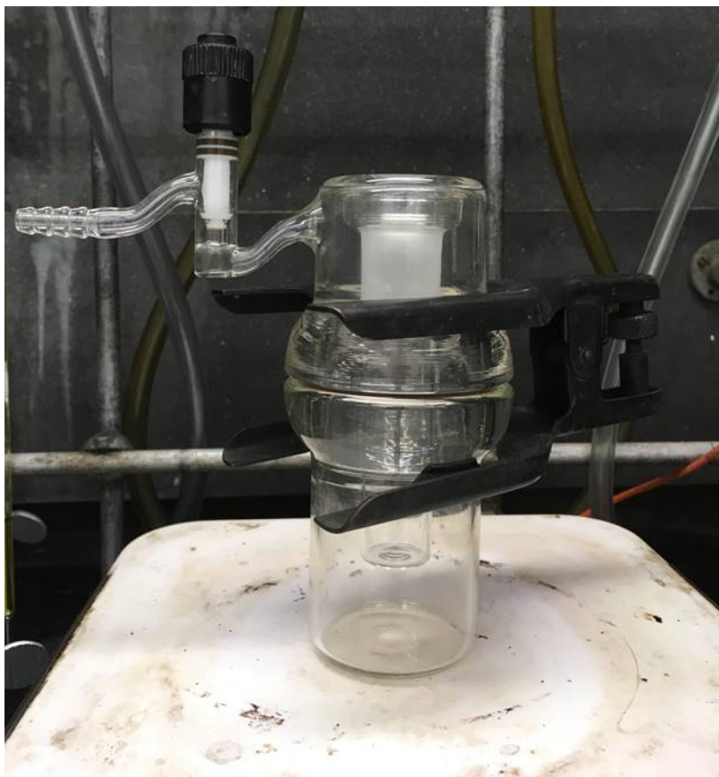
Figure 2. A sublimation chamber designed for low pressure sublimation.
