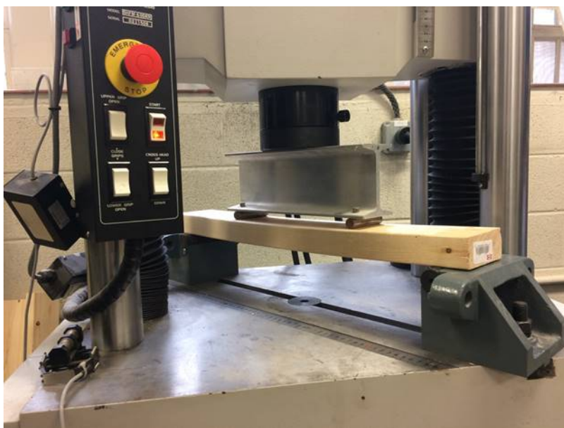
Figure 1: Four-point bending apparatus.
