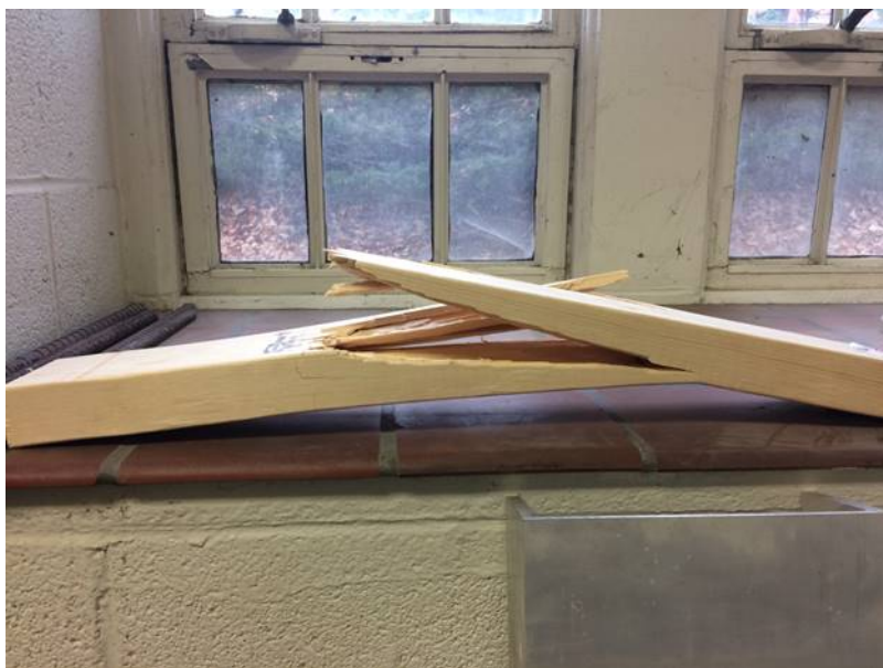
Figure 2: Wood beam flexural failure.
