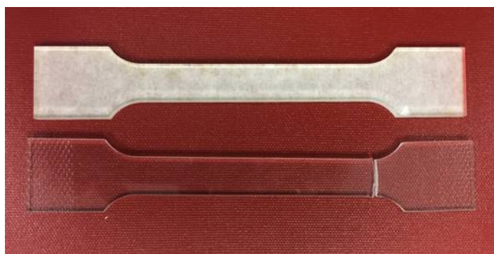
Figure 4: Failure in an acrylic specimen.
