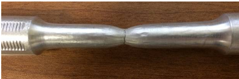
Figure 3 - Necking in aluminum specimen.
