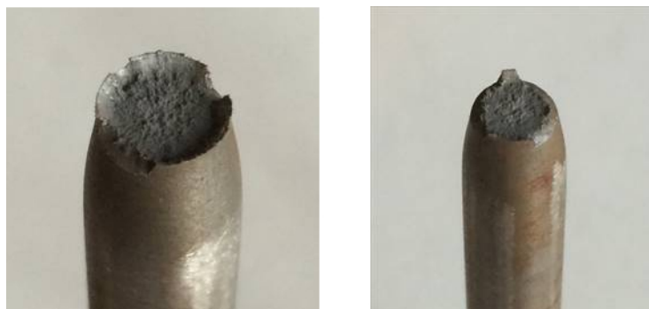
Figure 4: Typical ductile and brittle failure surface.
