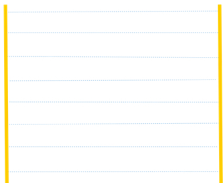
Figure 3: Diagram showing representative line patterns that may be formed by the powder, in the oil, aligning to the electric field produced by the charged electrodes corresponding to Figure 1 . The line patterns reflect the electric field lines and visualize the electric field.
