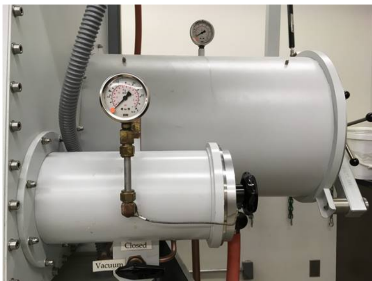
Figure 4. The large and small antechambers; each have their own pressure gauge and valve.
