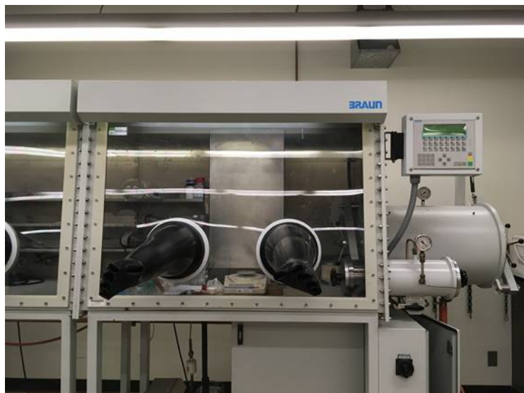
Figure 1. The glovebox, showing the main chamber, the gloves, the control panel, and the large/small antechambers. The gloves stick out when it is run at positive pressure.
