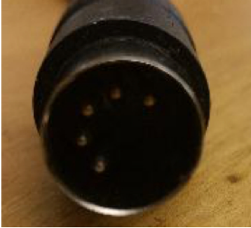
Figure 8: External power supply connector.
