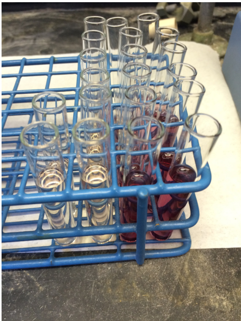
Figure 3. As the compounds elute off the column they are collected in test tubes. The compounds being separated in this experiment are colored, so they can be visually identified.
