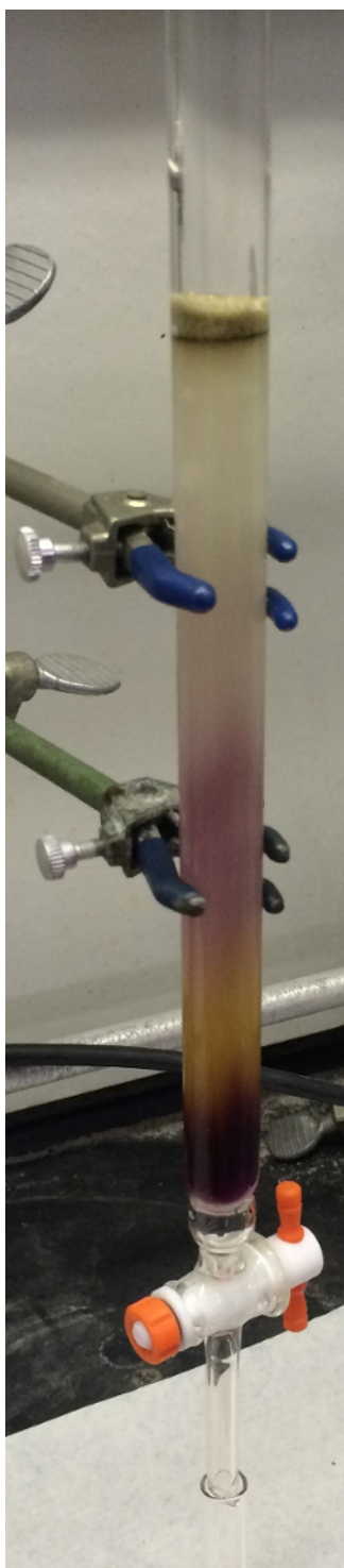
Figure 2. As the compounds traverse through the stationary phase they begin to separate. In this experiment the TPP (dark purple-reddish band) travels through the column slightly faster than the fluorenone (yellow band).
