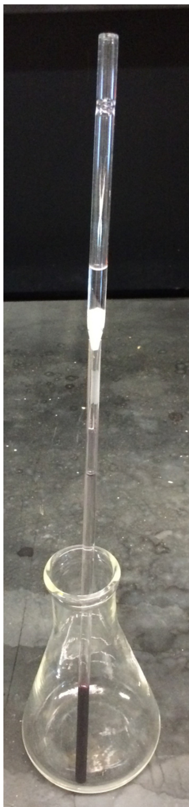
Figure 2. Once the solution containing targeted compound is placed in the crystal tube, the anti-solvent is slowly layered on top by passing it through a new pipette filter.
