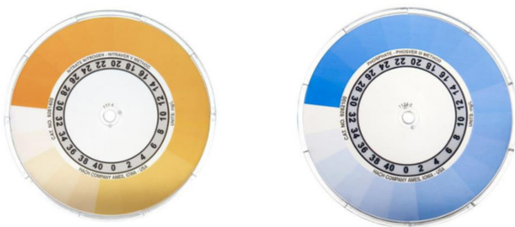
Figure 1. Example color disks for nitrate (left) and phosphate (right) color comparator boxes. Color intensities are on the outer edge of the disks and nutrient concentration (mg/L) are on the inner edge of the disks.
