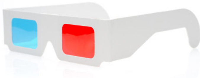
Figure 1. A pair of red-cyan rivalry glasses. The glasses make it possible to present two overlaid images such that only one arrives to each eye. The red lens will filter out all but red light before it reaches a viewer's eye, and the cyan lens will filter out all but blue light. This means that a blue tinted image won't make it to the eye with the red lens, and a red tinted image won't make it to the eye behind the blue lens.
