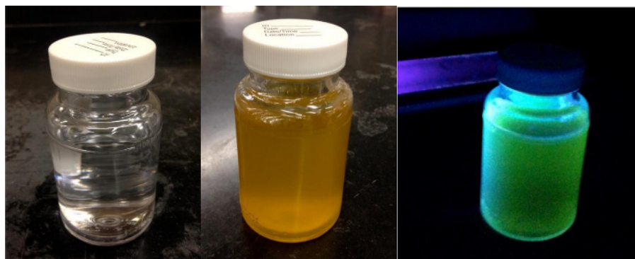
Figure 3. P-A test negative (left), coliform positive (middle), and E. coli positive (right).
